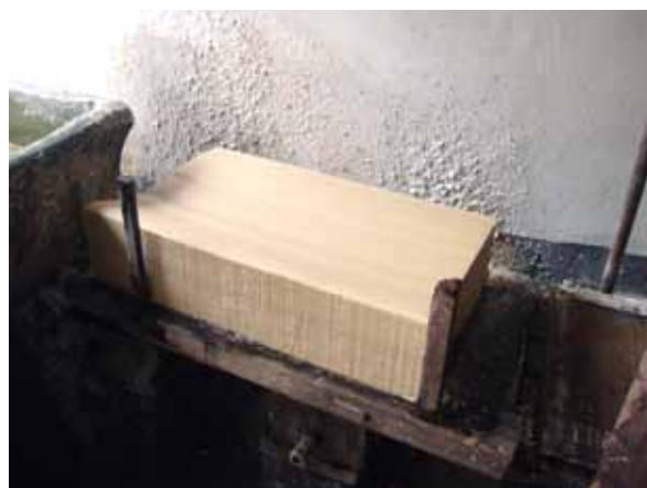
After each sheet is taken from the trough, it is stacked together and a heavy object is used to press out excess water.
