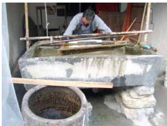
The thick pulp is placed in a stone trough, and water is added depending on the desired thickness.
